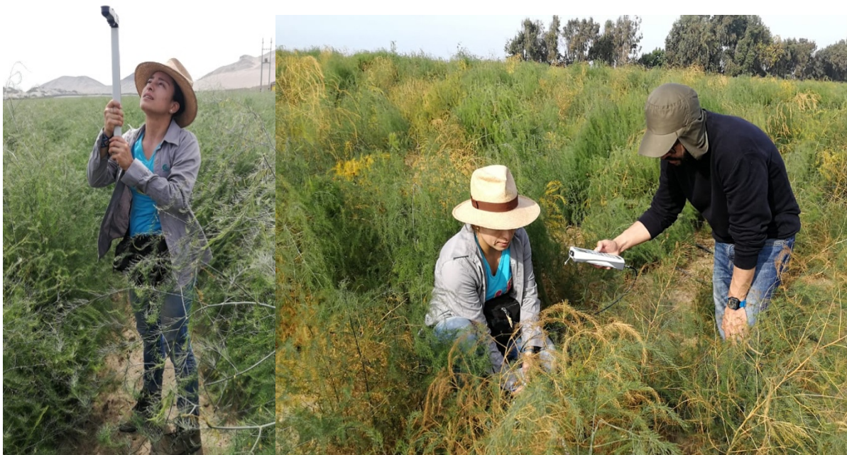
Figure 5. Taking light interception measurements using the LAI-2200C Plant Canopy Analyzer
