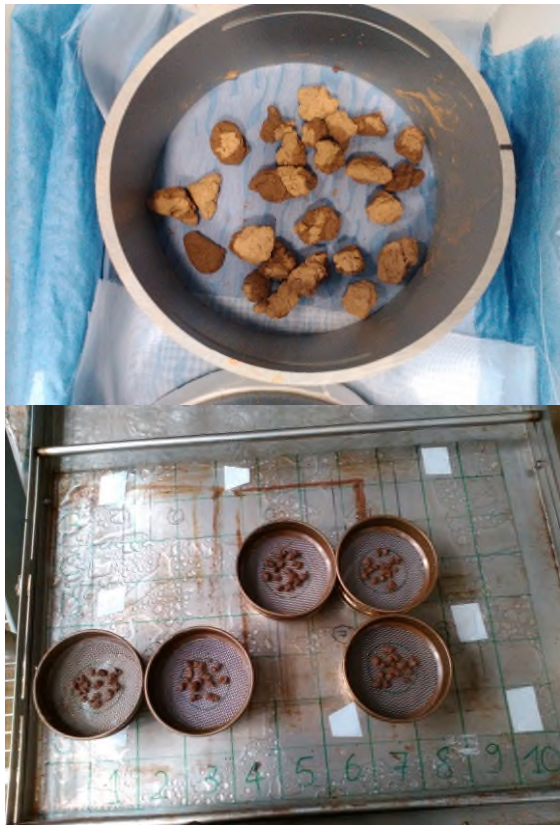
Aggregate stability test of the samples collected in November
