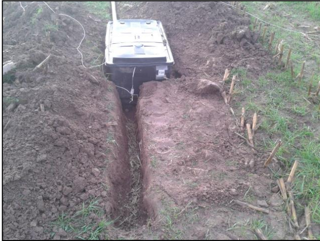
Figure 4. Instrumented storage tank and drain ditch.
