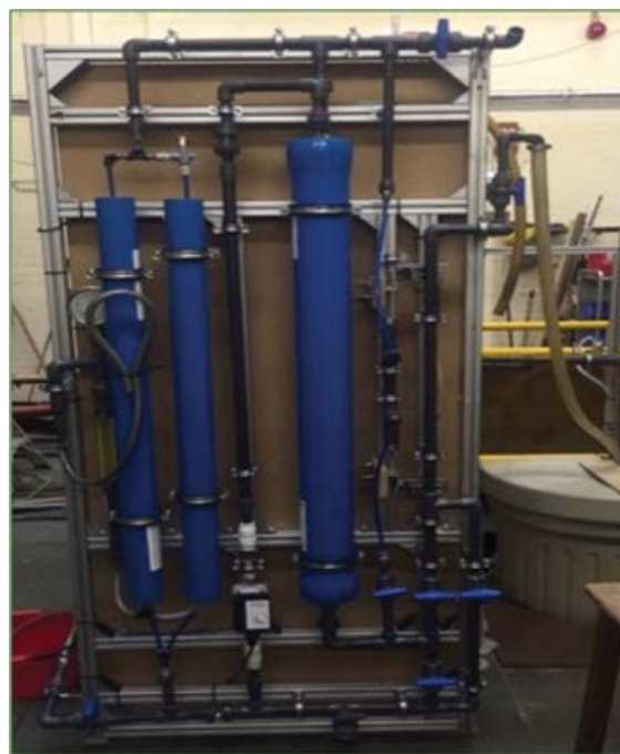
Fig. 2. Version 1 prototype: single-acting batch-RO system with manually operated valves, at Aston University, UK.
