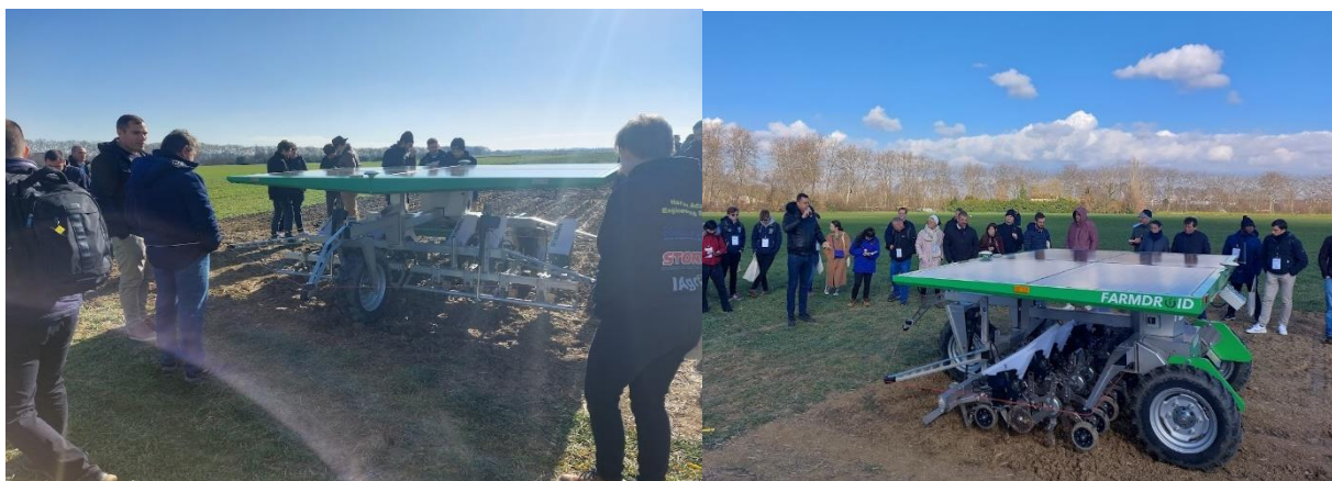
Figure 4 – Farm Driod – Autonomous weeding, cultivation and sowing unit reliant fully on solar power / batteries
