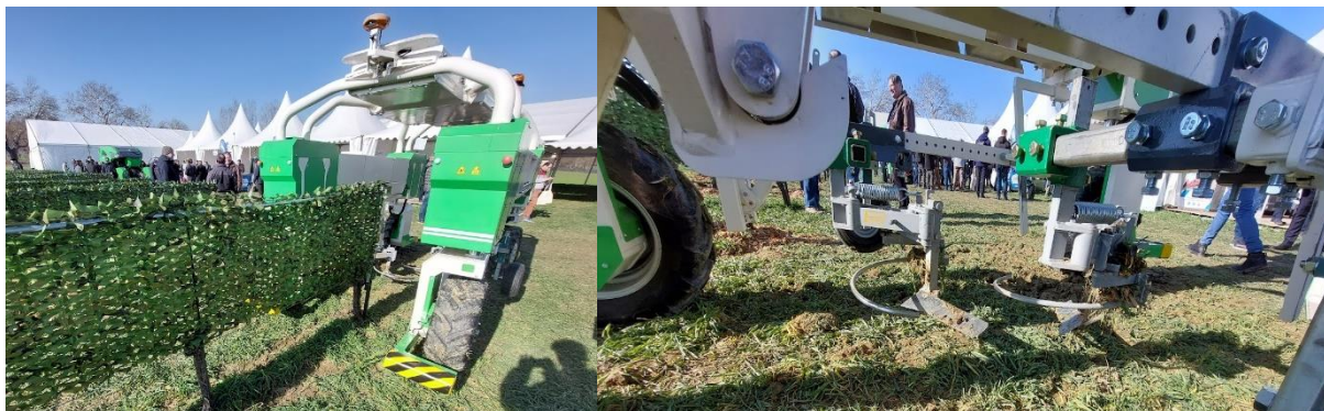
Figure 5 – Naïo Technologies vineyard tractor unit currently set up for intra-row vine weeding
